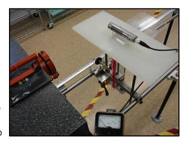
The instrument calibration laboratory is licensed to calibrate survey meters and dosimeters ranging from uR/hr to 10,000 R/hr using our Cs-137 range and box calibrators, and neutron survey meters and dosimeters ranging from 4 mrem/h to 20 mrem/h (ICRP 60) using our AmBe neutron calibrator. The laboratory also calibrates contamination monitoring equipment and provides detection efficiencies for most radioisotopes used in industrial, medical, and research applications.
